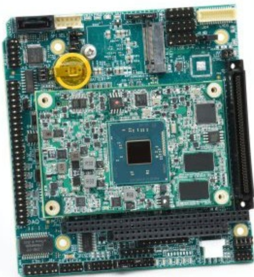
Athena IV baseboard with COM installed; heat sink removed for illustration purposes
