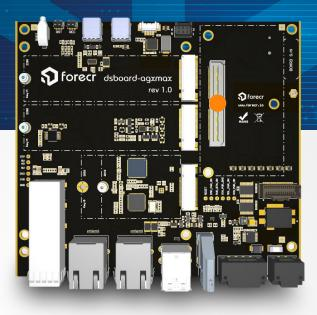
Introducing the DSBOARD-AGXMAX, the industrial carrier board that is built to maximize your productivity and connectivity. Powered by the high-performance AGX Orin SoM, which can deliver up to 275 TOPS of AI performance, this board offers top-of-the-line 10G connectivity, as well as Dual Gigabit Ethernet, USB 3.2, HDMI, CAN, Serial Ports, and MIPI CSI-2 Camera support.
