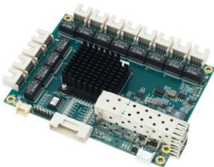
EPS-12G2 with 12 1G copper ports and 2 1G/2.5G SFP sockets
