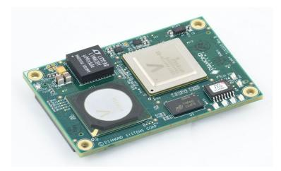
**EPSM-10GX Ethernet Switch Module**
