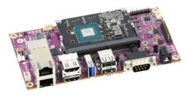
Floyd model BB01 with Nano module installed
