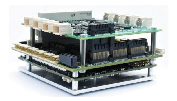
Gemini with PCIe/104 octal serial port module installed; 22mm board stacking height allows sufficient room for installed minicard + cabling
