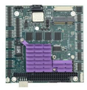
Helix "A" model with integrated data acquisition
