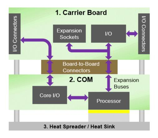
A COM-based SBC is a 2-board solution consisting of a Computer-on-Module (COM) that contains the processor and core I/O mounted on a carrier board that provides additional I/O and user connections. The carrier board brings out the I/O from the COM and provides additional I/O derived from the expansion buses provided by the COM, such as PCIE, LPC, SATA, and USB. This 2-board architecture provides significant advantages over traditional single-board computers.
