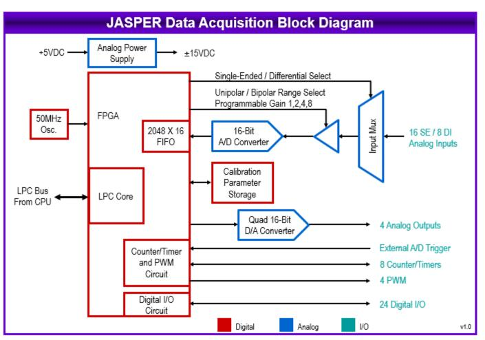
The A/D circuit includes 16 single-ended / 8 differential analog input channels with programmable input ranges and a maximum aggregate sampling rate of 250KHz. A built-in programmable counter/timer supports accurate high-speed sampling with precise timing. The 2048-sample FIFO with programmable threshold ensures error-free sampling and enables you to tune the performance of the circuit to minimize interrupt processing overhead.
