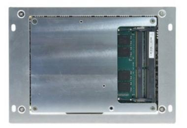
Jasper SBC bottom view showing mounting plate (outer) and COM heat spreader (inner)
