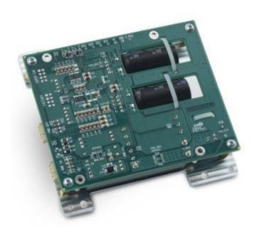
Assembly view with conduction cooling mounting plate
