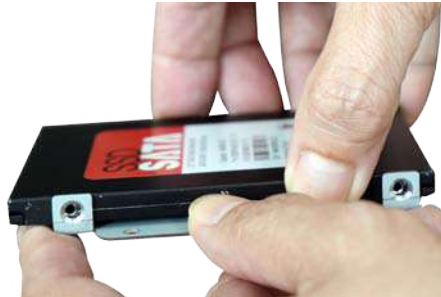
Install onto bracket
