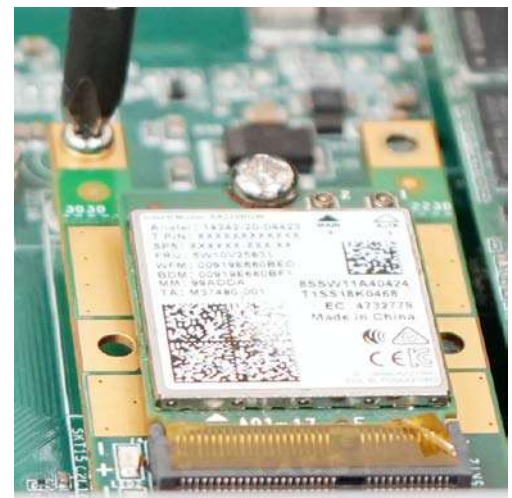
Secure using a screw
