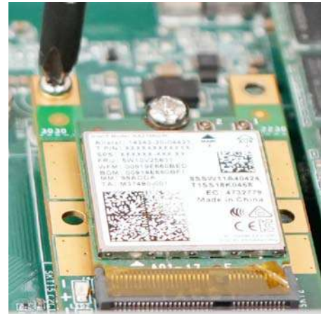
Secure using a screw
