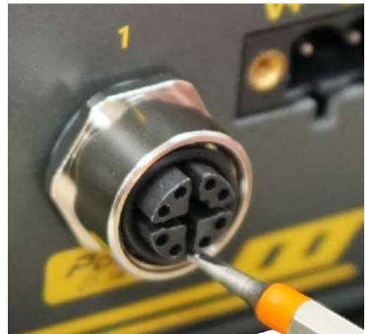
Tuck the O-ring into connector
