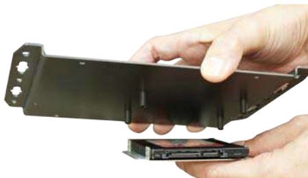
Install drive and bracket onto panel
