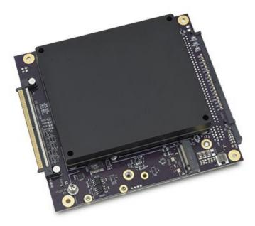
Osbourne with AGX Orin module installed
