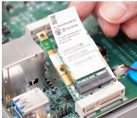
Insert on 45-degree angle
