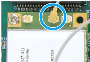
Clip on IPEX-to-SMA cable
