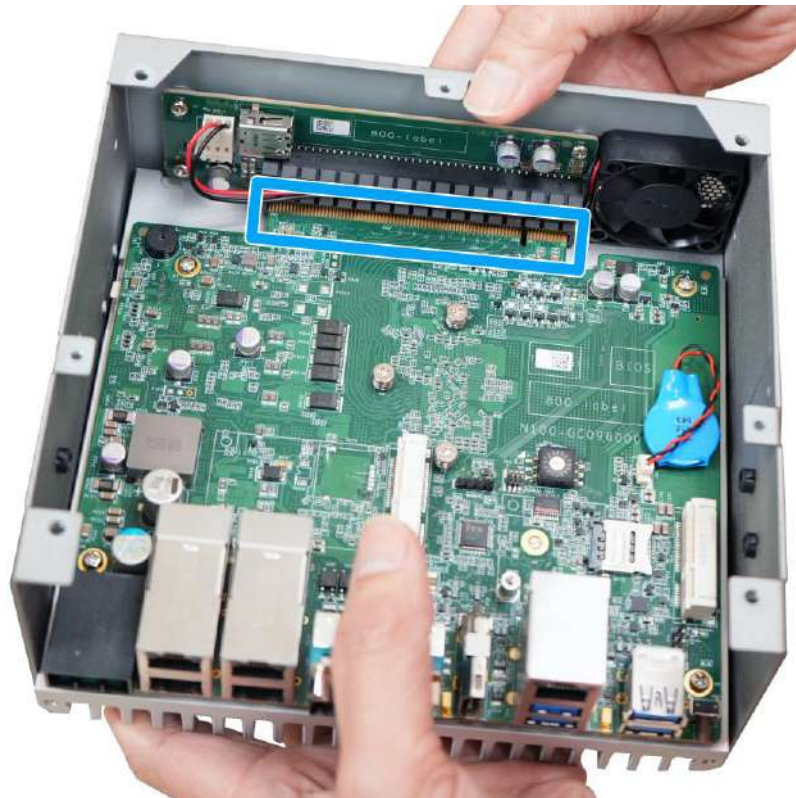
Properly insert into the PCIe slot
