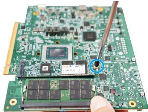
Secure with a P-head screw
