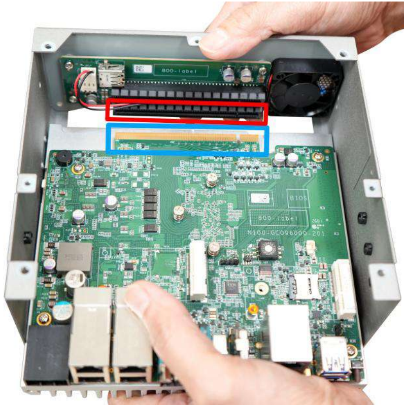
Matching the PCIe slot
