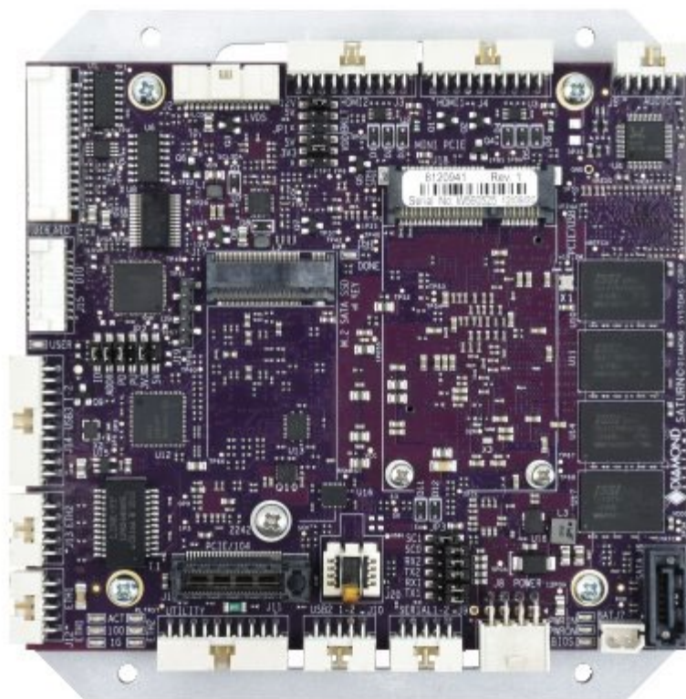
Saturn rugged SBC with E3940 CPU and data acquisition
