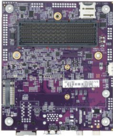
Module side with Xavier socket and M.2 socket
