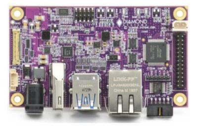
Ziggy Carrier for Jetson TX2/TX2i (2.0x3.4" / 50x87mm) Top View
