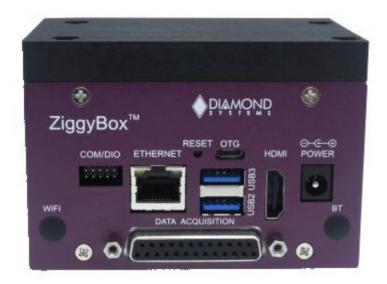
The ZiggyBox solution incorporates the Ziggy carrier board in a sturdy, miniature box. Everything needed for a complete system is provided in the ZiggyBox. Easy access connectors ensure data acquisition, Ethernet, HDMI, USB3.0 and USB2.0,WIFI, BT and COM/DIO are accessible. One side
