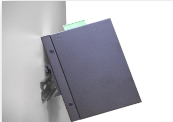
Figure 3.2 - Insert the Surge Protector on the DIN-Rail
